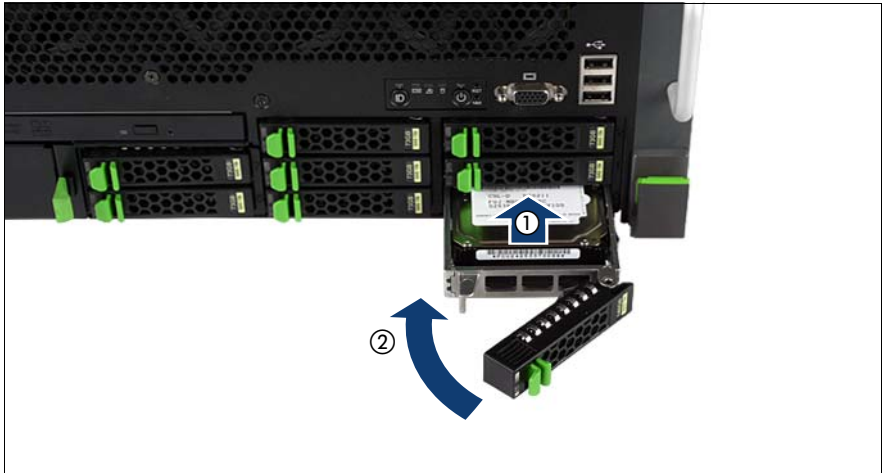
Figure 21: Installing the 2.5-inch HDD/SSD module
